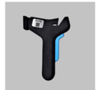
Model 701 Splice: ends opposed Range: up to 7000 tex Fibers: synthetics, glass, carbon, aramid, panox No cutting required
